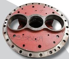
Original planet carrier with bearing journals which fall out of specification.
