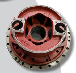
Original planet carrier with bearing journals which fall out of specification.
