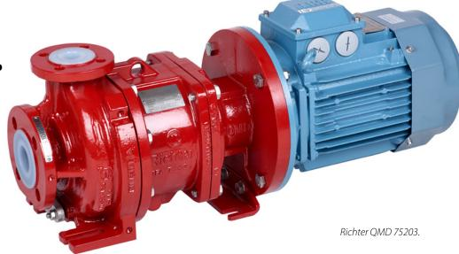
The pump series complies with the requirements of the local standard GB 5662, which can be equated with ISO 2858 and is designed for applications in the temperature range of -10°C to 100°C. The excellent chemical resistance provided by FEP lining and other high-quality materials such as silicon carbide, allows for flawless operation in applications with a performance range up to 125 m3/h and 65 m head.
