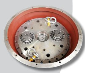
On completion - carriers with bearings and gears fitted inside the housings.
