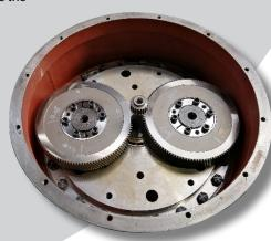
On completion carriers with bearings and gears fitted inside the housings.
